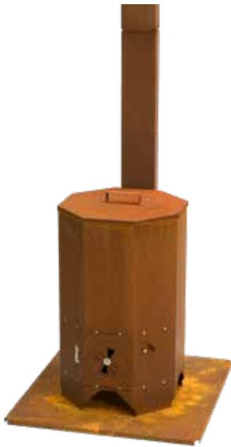
Separett Burn is a wood-fired stove for incinerating the dry waste from urine-separating toilets. The principle is based on the latrine bag from the urine-separating toilet being placed on a grating in the stove. Placed below the grating is wood which is then lit. In this way the bag with the dry waste is incinerated and only ash remains. The volume of wood used determines how good the incineration will be.
