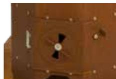
For combustion to be optimized adjust the air supply by turning the damper attached to the lower door.
