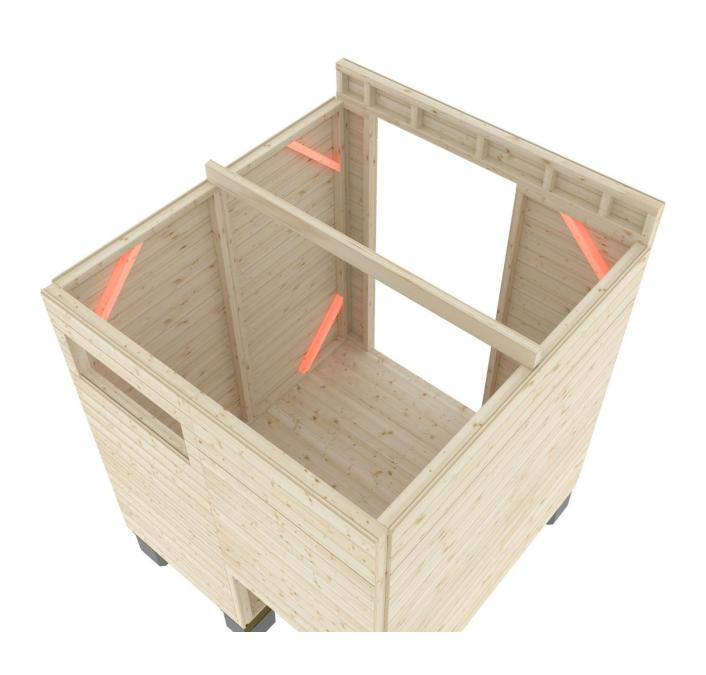
**8. THE ROOF BOARD INSTALLATION**. The roof board has slightly rounded edges on the front side and the back side is smooth. Roof boards are installed with the rounded side down, i.e. facing the cabin, and the smooth side up. Work carefully! Start nailing the roof from the low side. As with the floor, the last roof board should be split if necessary so that it ends even with the roof frame. 2 nails / ceiling beam are used for nailing. Roof boards seam is in the middle roof beam.
