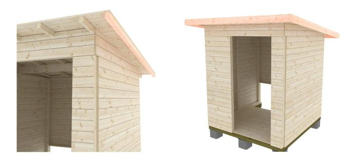
The wooden parts of the roof are finished with eaves and end boards, first you should install eaves boards that are same length as the roof board, so that the edges of the eaves board are even with the edges of the roofboards. The end boards come so that they cover the ends of the eavesboards. The eaves and end boards are nailed to the roof beams and side supports.
