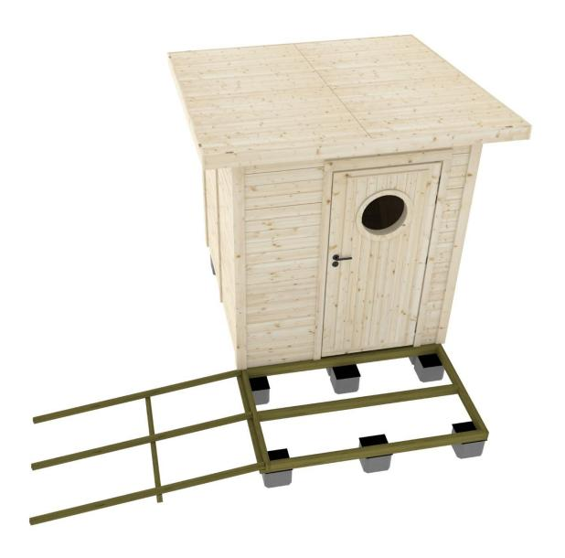
After frames are attached to foundation and cabin they can be finished with terrace board 21mm x 95mm. Ramp needs middle support as seen in picture below to prevent flexing.
