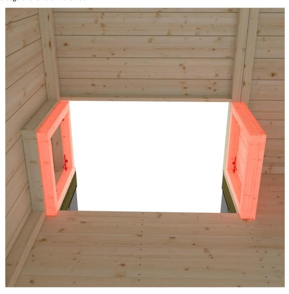
The seat element is lifted on the frames and and attached with screws (the side where the connecting board is even with the surface board is placed against the back wall) The front wall element is placed like a seat element with a screw-in frame.
