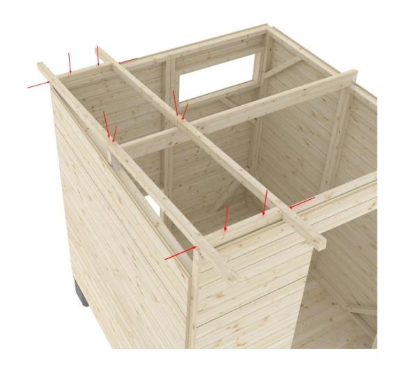
**6. FINISHING THE CLADDING** The end triangles are finished after the elements are installed. The paneling is continued from the top of the wall and over the roofbeam. The excess parts are sawed off with e.g. a hand saw, shown in red in the picture. In the same way, you can cover the intermediate timbers of the roof beams, in that case the panels should be split so that the upper part of the panel does not exceed the upper surface of the roof beam.
