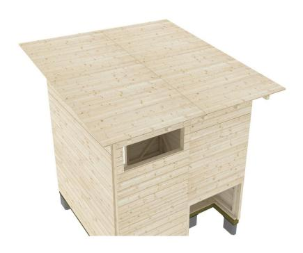
When the roof is boarded, the side supports are installed by screwing them from above through the roof board to the eaves. This makes it easier to attach the eaves and end boards.
