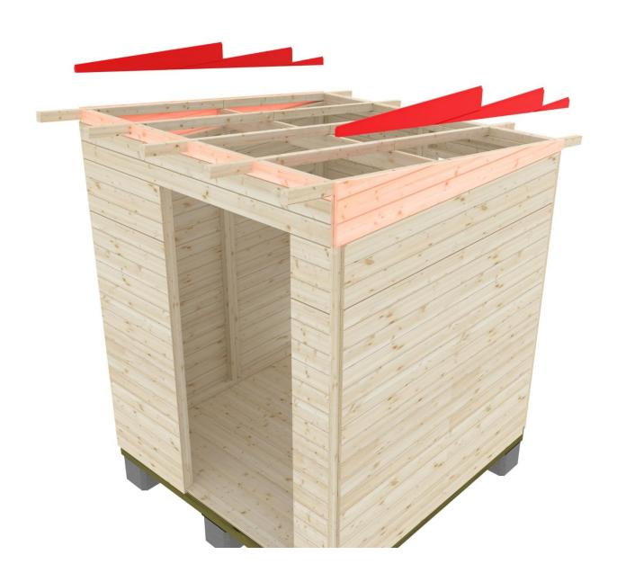
**7. DIAGONAL SUPPORTS** Before you start fixing the roof board, make sure that the walls of the cabin are straight. The delivery includes separately installed diagonal supports, it is recommended to install them at this stage.
