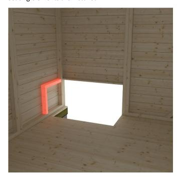
When the wall frame is folded, the frame of seating element is lifted into place, on the side of the wall and on the edge of the hole in the floor.
