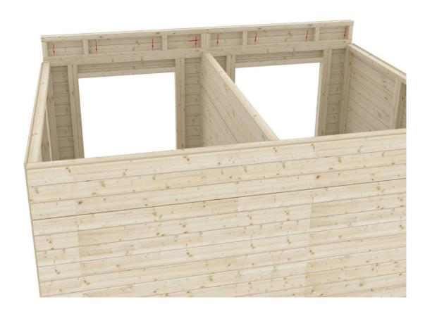
When the console elements are in place, its time to attach middle support for roof beams. Middle supports must be in the middle of the walls, and are attached by using angle irons. Middle supports consists of two pieces. joint is placed in the middle of the wall between the toilets.
