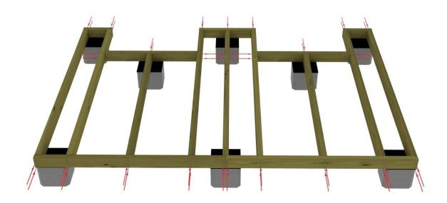
**3. FLOORING** The installation of the floor starts by placing the floorboard on the baseboards with the bevels down and the side with slot facing the outer edge. Nail the floorboards into place one at a time. The floorboard is installed before the outer walls. The outer walls are installed on top of the floorboards. The last floorboard should be sawed so that the edge is even with the subframe. The floor should be protected from dirt immediately after installation.
