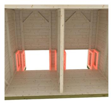
The seat element is lifted on the frames and a attached with screws (the side where the connecting board is even with the surface board is placed against the back wall) The front wall element is placed like a seat element with a screw-in frame.
