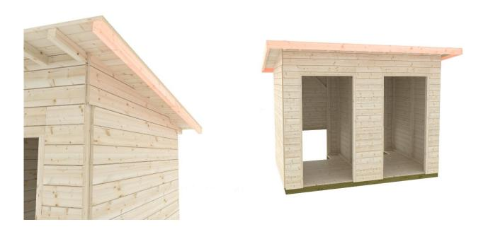
The wooden parts of the roof are finished with eaves and end boards, first you should install aa eaves boards that are same length as the roof board, so that the edges of the eaves board are even with the edges of the roof board. The end boards come so that they cover the ends of the eaves boards. The eaves and end boards are nailed to the roof beams and side supports.
