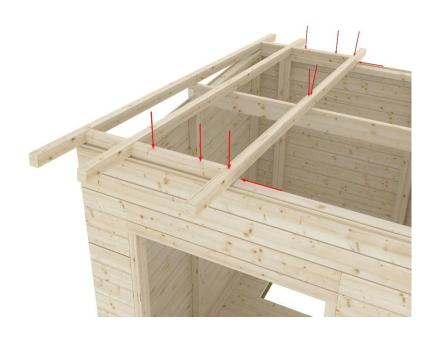
**7. FINISHING THE CLADDING** The end triangles are finished after the elements are installed. The paneling is continued from the top of the wall element. After paneling, the excess parts are sawed off with e.g. a hand saw, shown in red in the picture. In the same way, you can cover the intermediate timbers of the roof beams, in that case the panels should be split so that the upper part of the panel does not exceed the upper surface of the roof beam.
