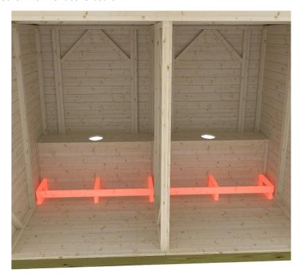
After that step element is lifted on frames and screwd in place.
