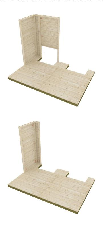
**5. WALL BETWEEN TWO TOILETS**, before installing elements panel at the bottom should be sawed to the same level as bottom of the frame. That way wall elements will stand on its frame and will be leveled with rest of the walls. Its very important that both toilets are have same width, so seat element would fit when its time to place them.
