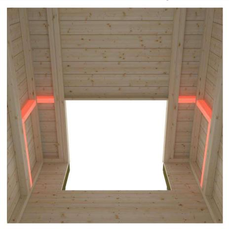
When the wall frame is folded, the frame of seating element is lifted into place, on the side of the wall and on the edge of the hole floors hole.
