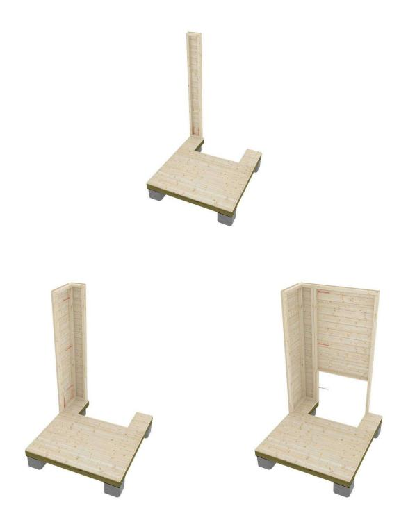
Fasten the elements together with about three screws. Also fasten the elements to the subframe. See the arrangement of the elements in the element diagram or the floor plan.
