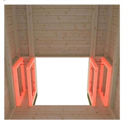
The seat element is lifted on the frames and a attached with screws (the side where the connecting board is even with the surface board is placed against the back wall)
