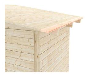
When the roof is boarded, the side supports are installed by screwing them from above through the roof board to the eaves. This makes it easier to attach the eaves and end boards.
