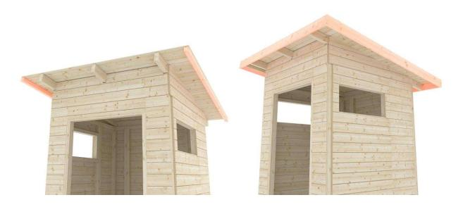
The wooden parts of the roof are finished with eaves and end boards, first you should install aa eaves boards that are same length as the roof board, so that the edges of the eaves board are even with the edges of the roof board. The end boards come so that they cover the ends of the eaves boards. The eaves and end boards are nailed to the roof beams and side supports
