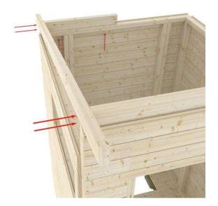
When the console elements are in place, the installation of the roof frame begins. The first roof beam is installed right on the edge of the frame, followed by an intermediate block between the roof beams, which is screwed through the upper part of the element. Outer roof beam can then be screwed from the side to the intermediate block.
